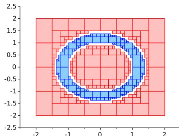
**Remark:** involving bisection algorithm and so complexity is exponential in the size of the state space (contractor programming to overcome this).
